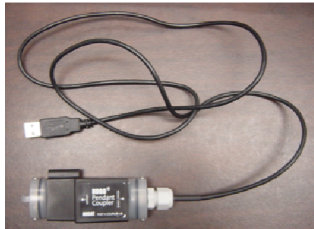
Figure 1: USB HOBOWare base station
